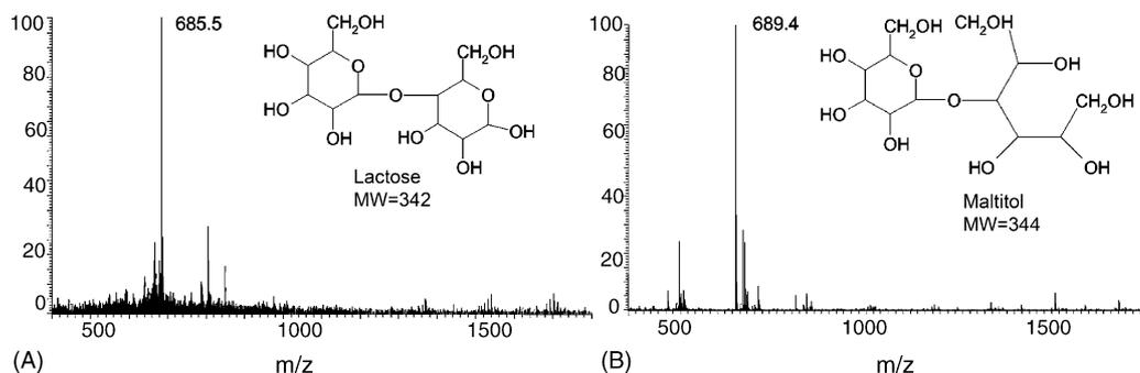
Fig. 1. Gradient tracer molecules. The characteristic mass spectrum for the gradient tracer molecules (A) lactose and (B) maltitol.
