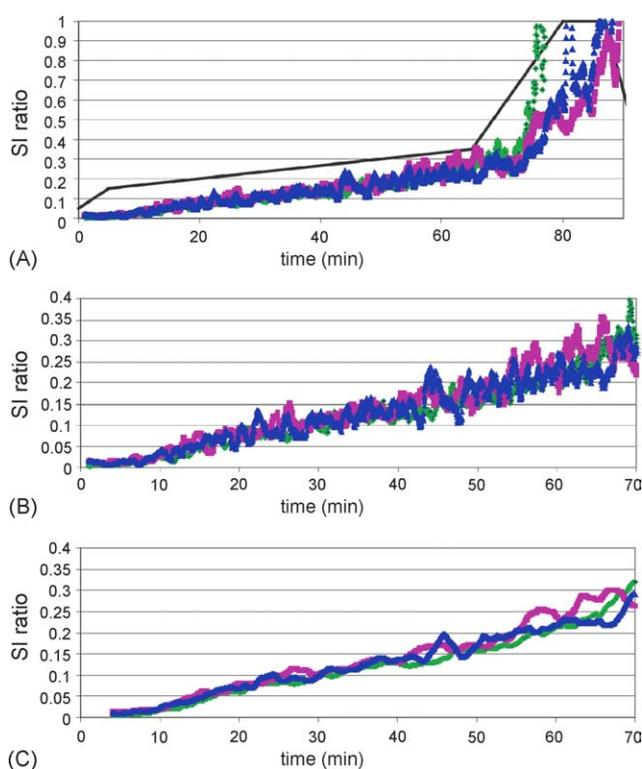
Fig. 5. Run-to-run reproducibility of SI-ratio for three runs using gradient 1. (A) Chromatogram of entire 90 min run. (B) SI-ratio during the typical peptide elution range. (C) SI-ratio with signal-to-noise smoothing.
