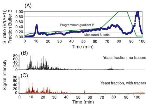
Fig. 4. Simultaneous LC-gradient monitoring and MS/MS based peptide sequence identification from yeast. Using LC gradient 1 as described (A) we identified 300 high-scoring peptide sequences in the yeast fraction without tracers (B) and 320 high-scoring peptide sequences in the yeast fraction with tracers (C). We were also able to follow the gradient using the SI-ratio while acquiring CID-spectra of these yeast peptides (A).
